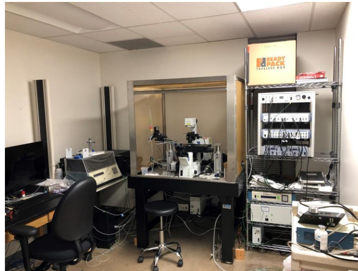
4-laser confocal microscope with automated stage, 2 e-phys channels and calcium imaging
